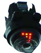
LED fault indicators use improved technology to reduce outage time.
