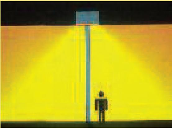
This diagram shows the effect of dark-sky friendly lighting. You can see there is no light shining toward the sky and there is essentially no glare. Virtually all of the light is aimed downward where it is needed. (Note: The light in the picture here is only an example and is not a light style that is currently available from NOVEC.)
